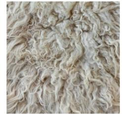
Flinders University scientists have developed a new composite made of waste cooking oil, sulphur and wool offcuts to produce a sustainable housing insulation material. The product is now being commercialised by Clean Earth Technologies. Capitalising on wool's natural low flammability, the new composite is yet another application for a polymer that was initially developed to retrieve oil after a large-scale spill.
