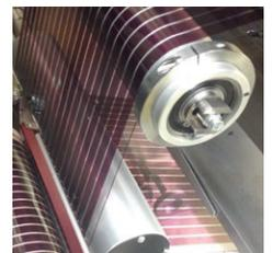
ANFF Materials at the University of Newcastle is supporting the development of a printed solar cell technology that could revolutionise energy capture. Hundreds of metres of the team's solar sheets can be printed per day using a photovoltaic ink, polymer substrate, and roll-to-roll printing techniques found in the printing industry.
